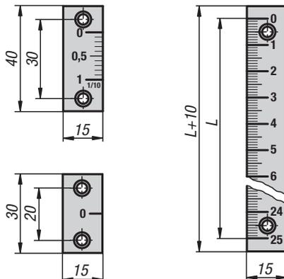
Black anodized surface and high contrast graduations for legibility without shading. The graduations are deep lasered.
