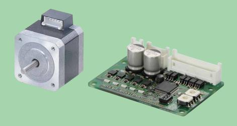
Revisions to the motor winding design and a high-efficiency driver circuit design allow for significant torque increases in the low-speed range. In particular, torque in the 250 r/min range has been increased by 50% compared to conventional products allowing for quicker moves. Vibration and noise have been greatly reduced compared to conventional 1.8° stepper motor performance.
