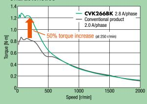
The maximum holding torque has increased with a bipolar winding.
