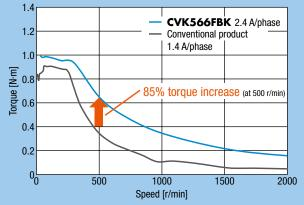
By adopting a higher current motor winding specification, the usage range is now much wider.
