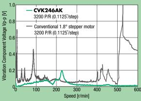
The vibration characteristics have been significantly improved across all speed ranges with the fully digital-controlled microstep driver.
