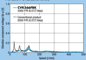
Lower vibration and further noise reductions have been achieved through the use of a fully digital-controlled microstep driver.
